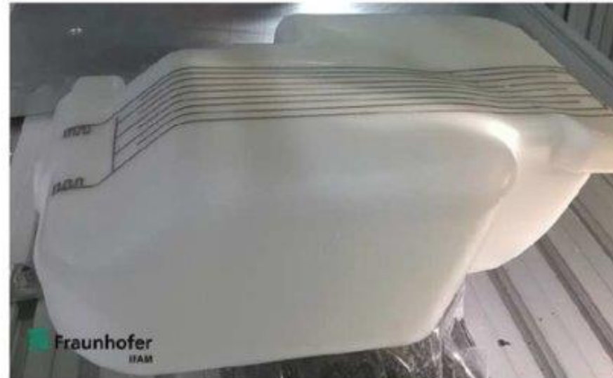
Printed capacitive filling sensor on 3D-Object
